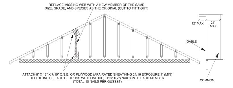
THE OUTSIDE FACE OF THE GABLE MUST BE SHEATHED WITH (MIN) 7/16" O.S.B OR PLYWOOD. SEE MITEK STANDARD GABLE END DETAILS FOR WIND BRACING REQUIREMENTS.
