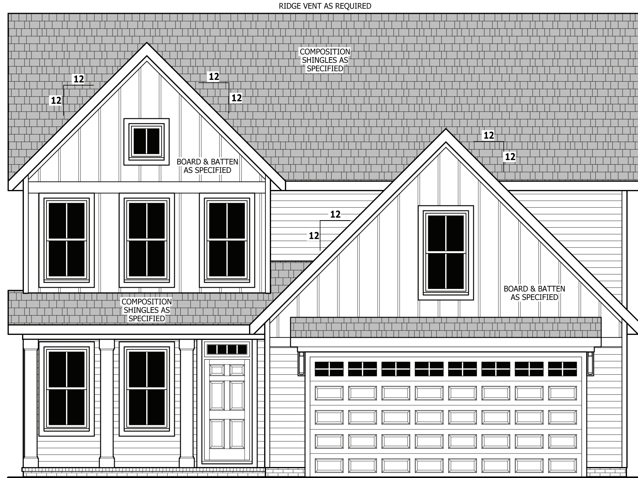
FRONT ELEVATION - B SCALE 1/4" = 1'-0"
