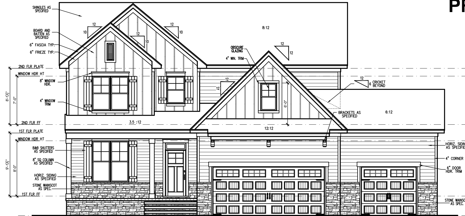
FRONT ELEVATION 'B' - 3 CAR FRONT LOAD (CRAWL) SCALE: 1/8"=1'-0" ON 11x17, 1/4"=1'-0" ON 22x34
