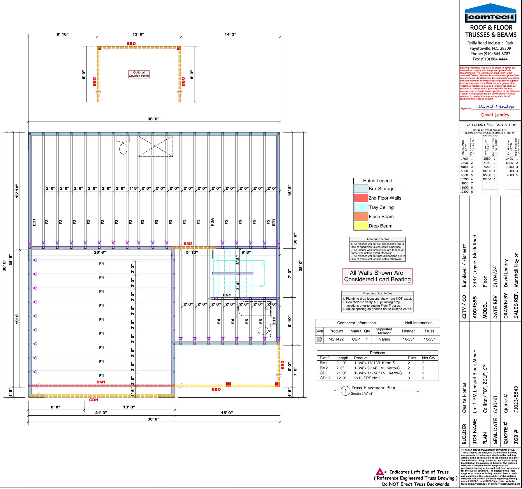
**A** = Indicates Left End of Truss (Reference Engineered Truss Drawing) Do NOT Erect Truss Backwards
