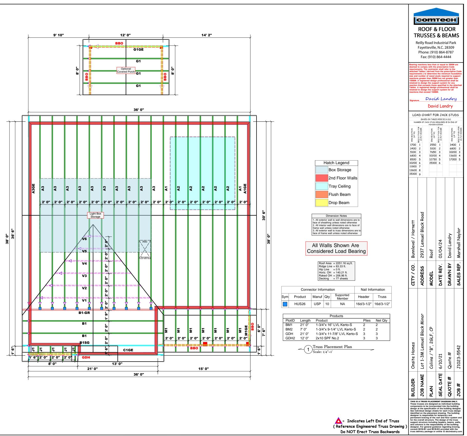
▲ = Indicates Left End of Truss (Reference Engineered Truss Drawing) Do NOT Erect Truss Backwards
