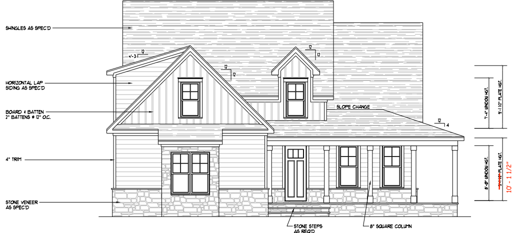
FRONT ELEVATION "A" SCALE: 3/16" = 1'-0"
