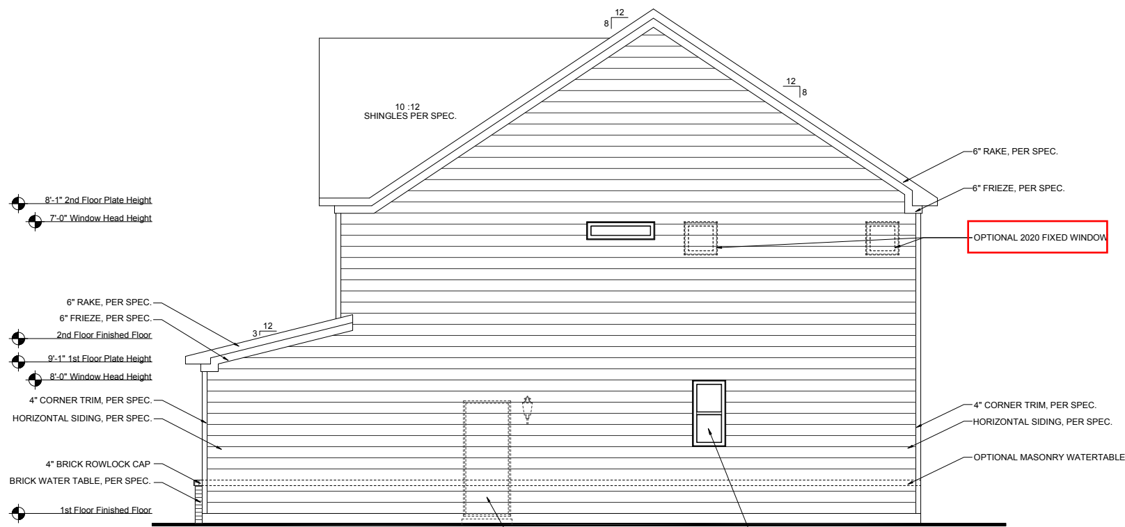
WILLOW RIGHT ELEVATION - 'B' SCALE: 1/8"=1'-0" (11"X17" SHEET SIZE) SCALE: 1/4"=1'-0" (22"X34" SHEET SIZE)
