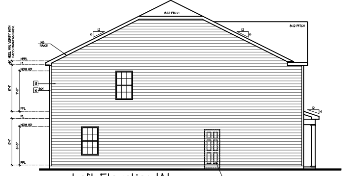
Left Elevation 'A' SCALE: 1/4"=1'-0" AT 22'X34" LAYOUT 1/8"=1'-0" AT 11'X11" LAYOUT
