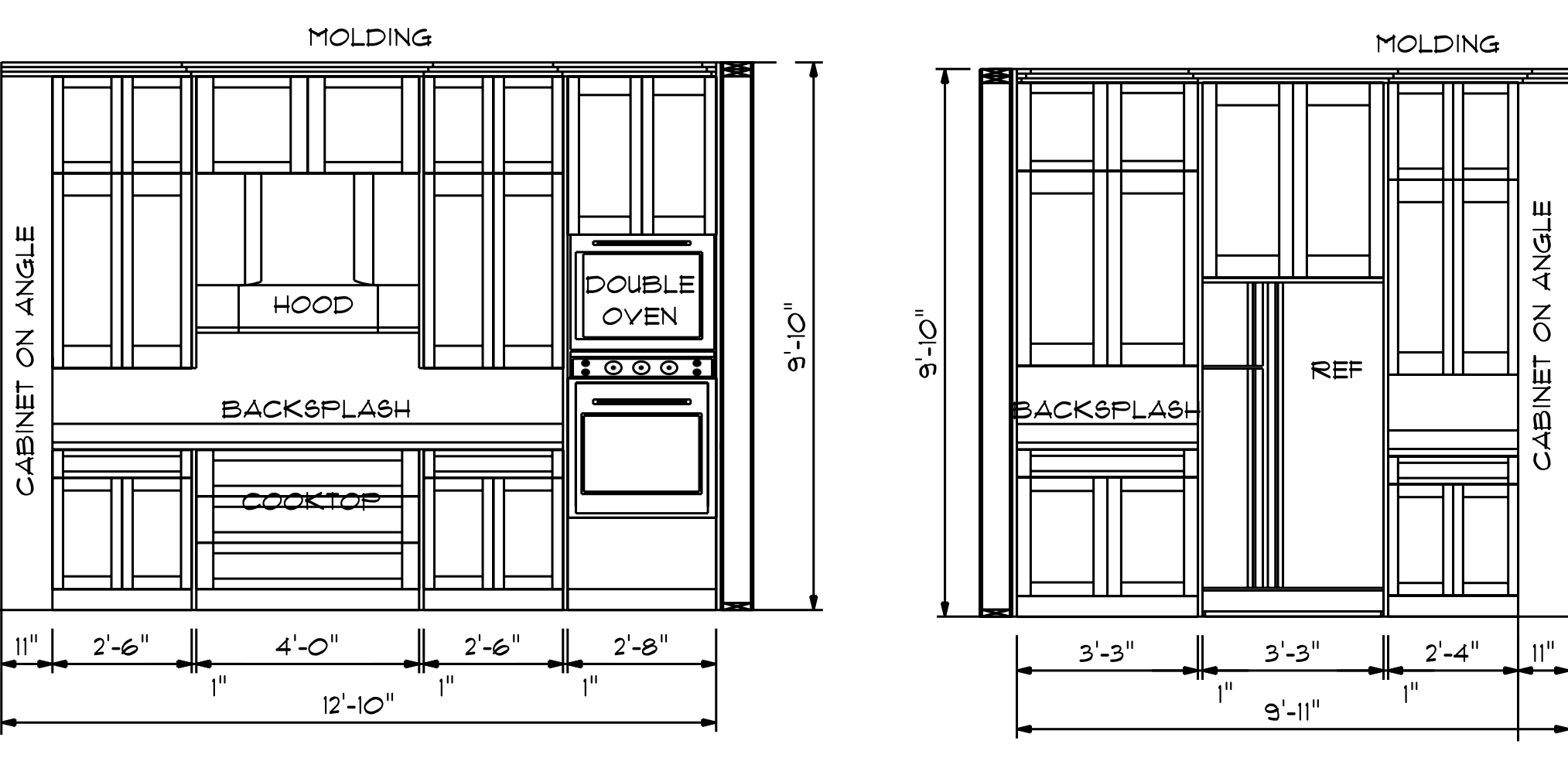
KITCHEN CABINET ELEVATIONS SCALE: 3/8" = 10"
