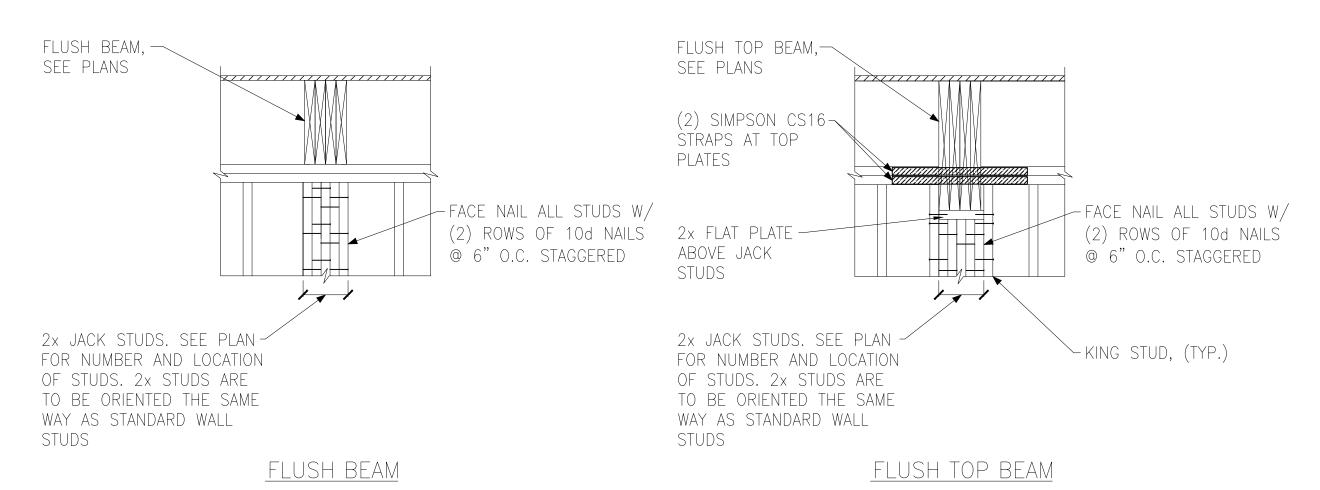
BUILT-UP STUD DETAIL SUPPORTING BEAM
