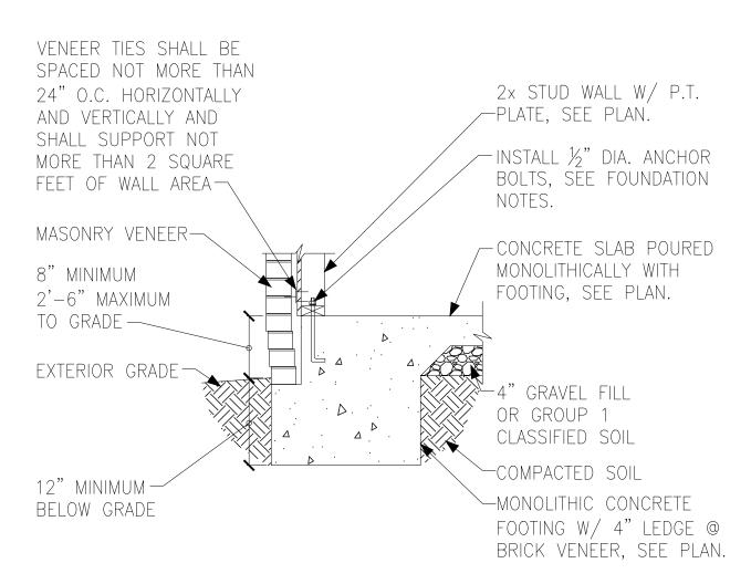
FOUNDATION SECTION B) EXTERIOR WALL @ MASONRY VENEER
