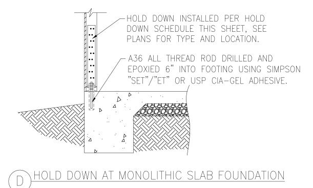
HOLD DOWN INSTALLED PER HOLD DOWN SCHEDULE THIS SHEET, SEE PLANS FOR TYPE AND LOCATION. \_ A36 ALL THREAD ROD DRILLED AND EPOXIED 6" INTO FOOTING USING SIMPSON "SET"/"ET" OR USP CIA-GEL ADHESIVE.
