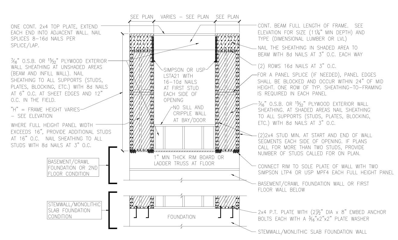
\METHOD CS-PF: CONTINUOUS PORTAL FRAME PANEL CONSTRUCTION B)TWO BRACED WALL SEGMENTS
