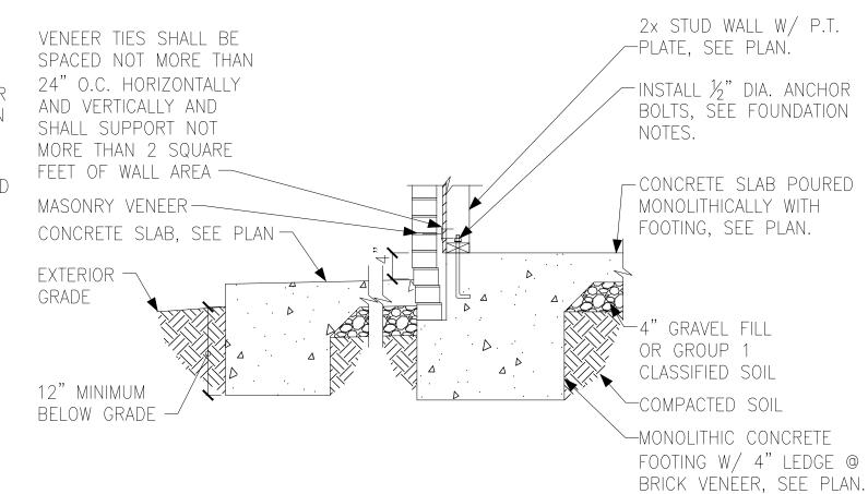
\FOUNDATION SECTION /EXTERIOR WALL AT PORCH W/ MASONRY VENEER
