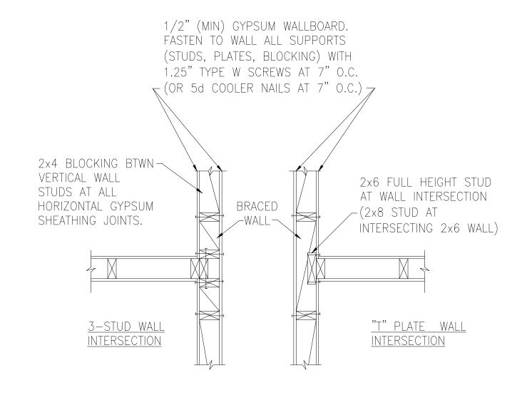
BRACED WALL INTERSECTIONS MAY BE FRAMED USING EITHER THE 3-STUD OR THE T-PLATE METHOD.
