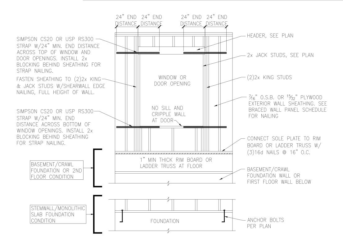
WINDOW OR DOOR REINFORCEMENT IN ENGINEERED SHEAR WALL ONLY REQUIRED WHERE SPECIFED ON PLANS
