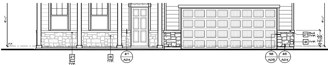
PARTIAL FRONT ELEVATION 'D' W/ MASONRY OPTION AT 9'-0" PLT. HGT. SCALE 1/4"=1'-0" (22"X34") - 1/8"=1'-0" (11"X17")
