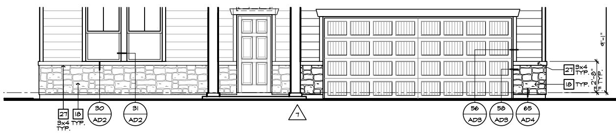
PARTIAL FRONT ELEVATION 'B' W/ MASONRY OPTION AT 9'-0" PLT. HGT. SCALE 1/4"=1'-0" (22'x34") - 1/8"=1'-0" (11'x17")
