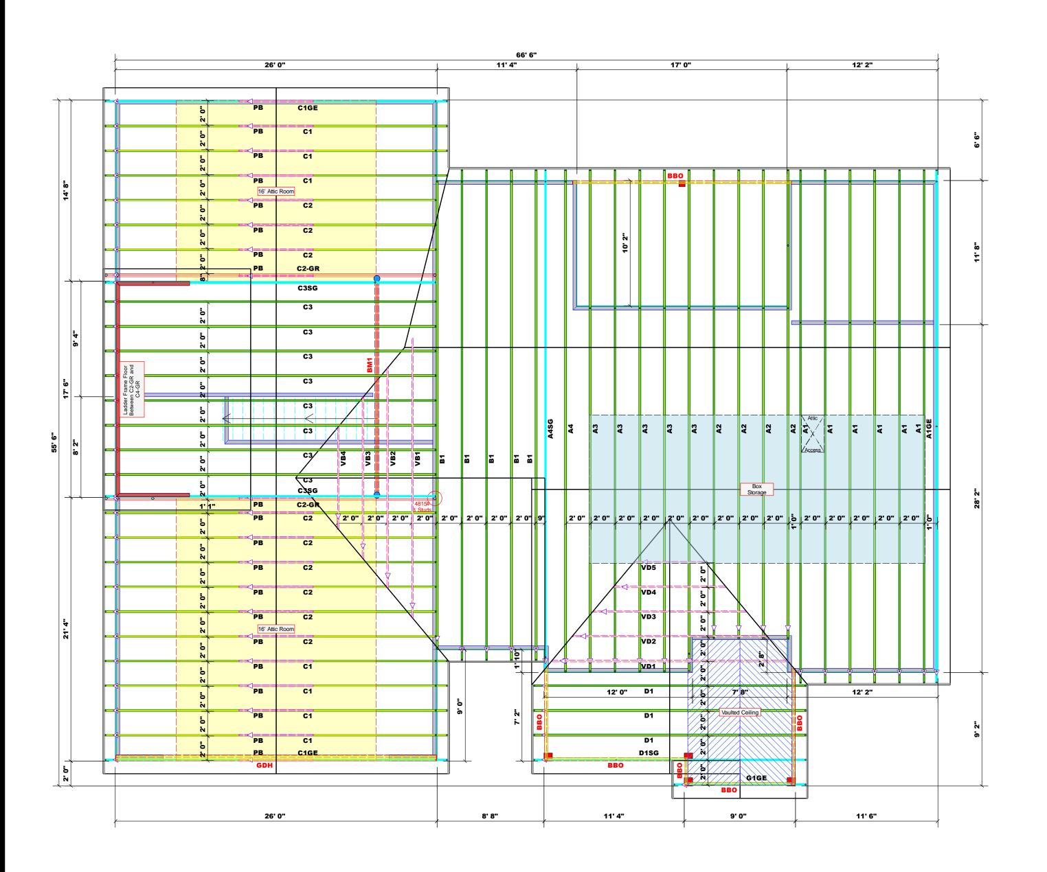
All Truss Reactions are Less than 3,000 lbs. Unless Noted Otherwise. - Denotes Reaction Greater than 3,000 lbs. Reaction / # of Studs
