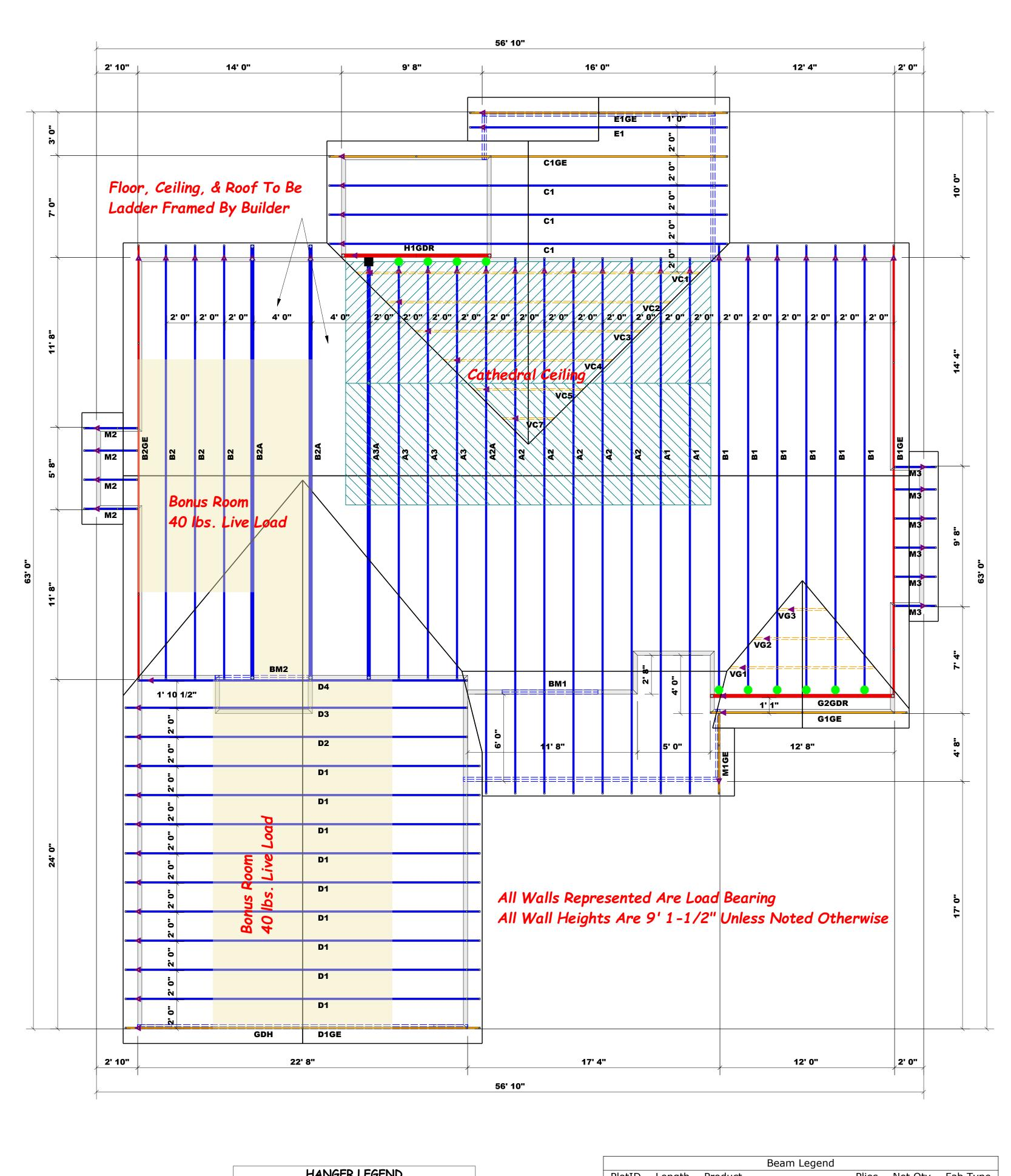
▲ = Denotes Left End of Truss (Reference Engineered Truss Drawing) Do Not Erect Trusses Backwards
