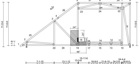
Repair for a section of the verticals missing above joi t 18.
