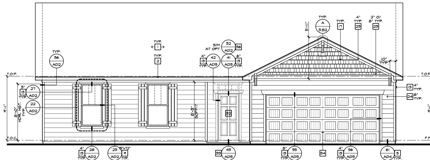
FRONT ELEVATION 'B' AT OPTIONAL 9'-1" PLT. HGT.
