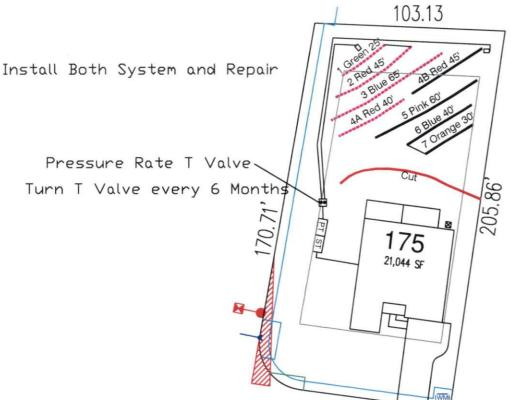
System: Pressure Manifold Lines: 1-4A, (175') T&J Panel 50% Reduction 0.3 Soil LTAR 22" Trench Bottom
