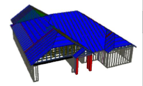
THE PURPOSE OF THIS DETAIL IS TO ILLUSTRATE HOW TO PROPERLY SPACE 24" O.C. ROOF TRUSSES TO ALLOW FOR A 25 1/2" OPENING FOR PULL DOWN ATTIC ACCESS
