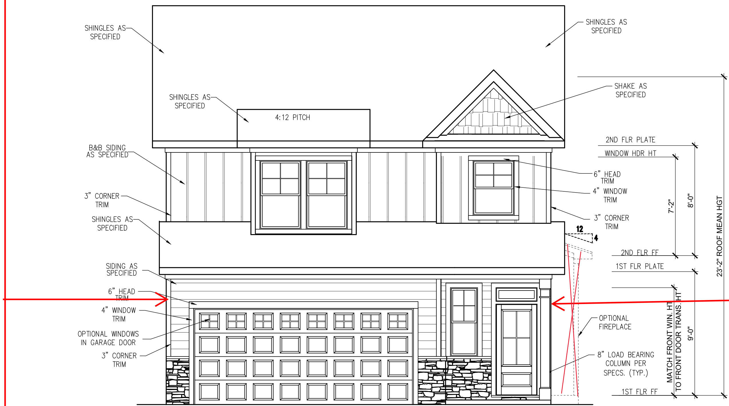
OPTIONAL FRONT ELEVATION FRENCH COUNTRY - 3 BEDROOM - (SLAB) SCALE: 1/4" = 1'-0" ON 22x34, 1/8" = 1'-0" ON 11x17
