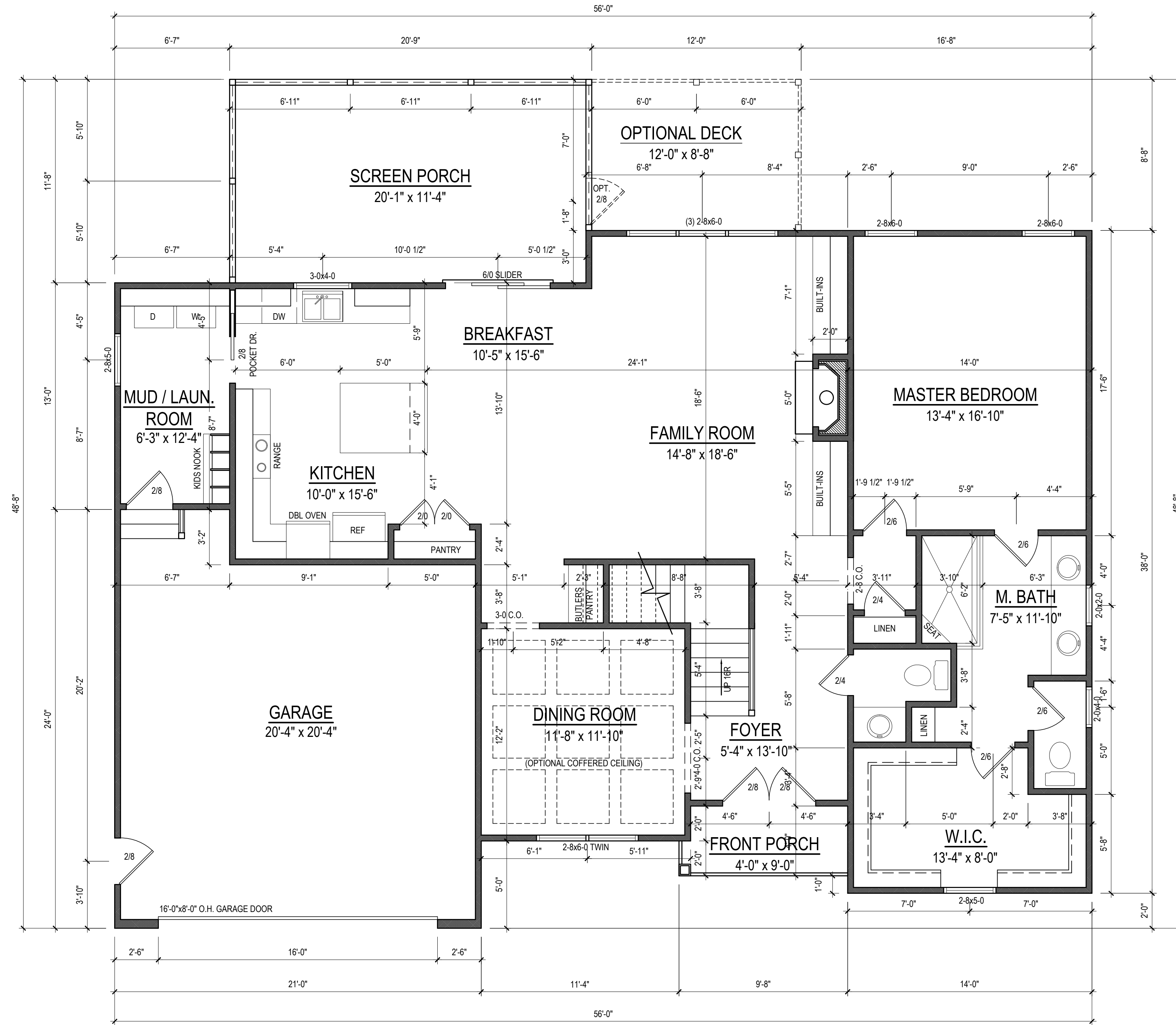
FIRST FLOOR PLAN 1/4" = 1'-0" CEILING HT. = 9'-0"
