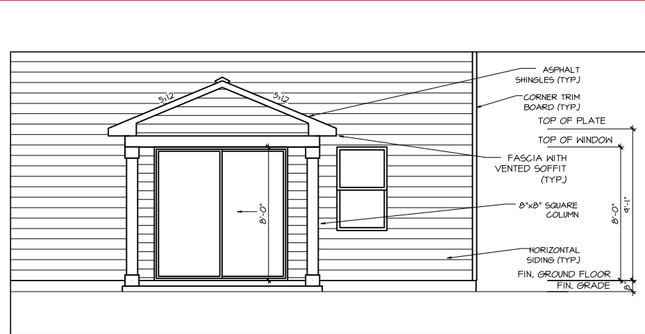
COVERED VERANDA PPO - REAR ELEVATION
