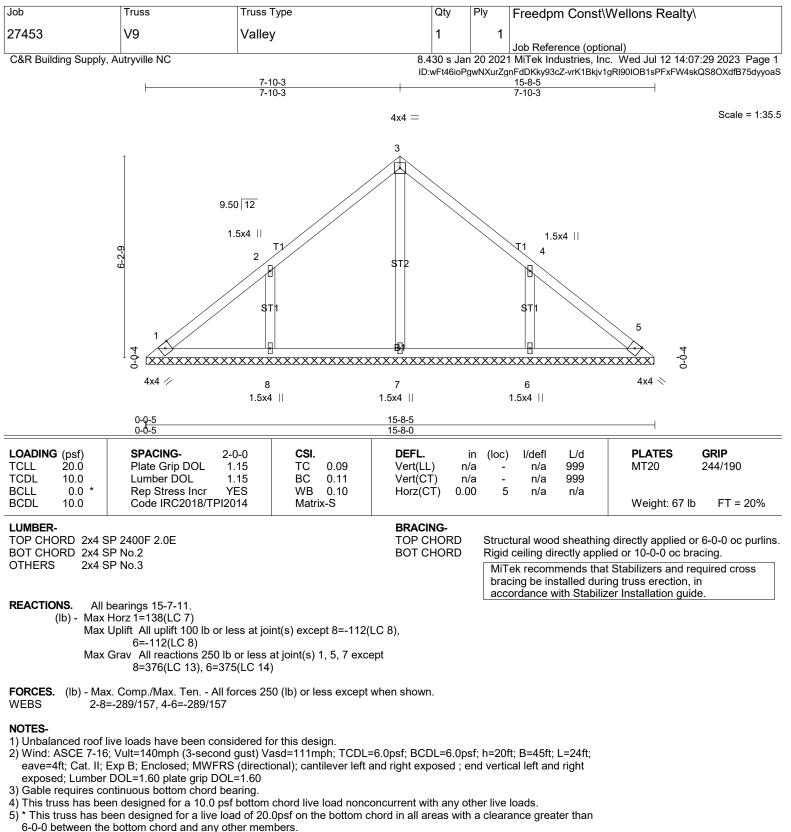
6) Provide mechanical connection (by others) of truss to bearing plate capable of withstanding 112 lb uplift at joint 8 and 112 lb uplift at joint 6.
