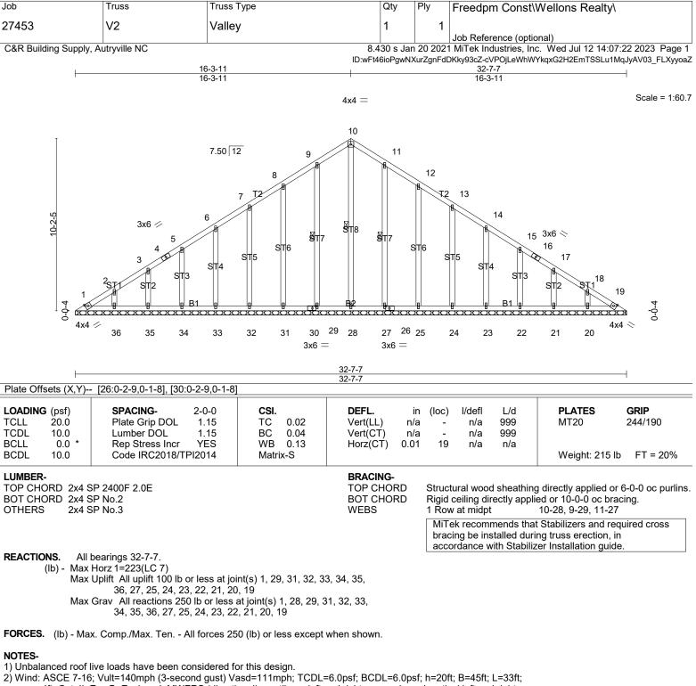
eave=4ft; Cat. II; Exp B; Enclosed; MWFRS (directional); cantilever left and right exposed ; end vertical left and right exposed; Lumber DOL=1.60 plate grip DOL=1.60
