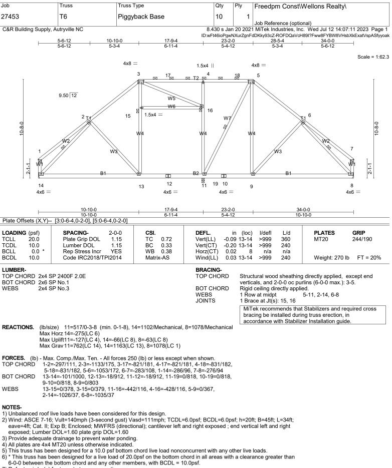
7) Refer to girder(s) for truss to truss connections.
