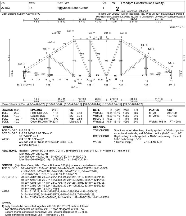
2) All loads are considered equally applied to all plies, except if noted as front (F) or back (B) face in the LOAD CASE(S)
