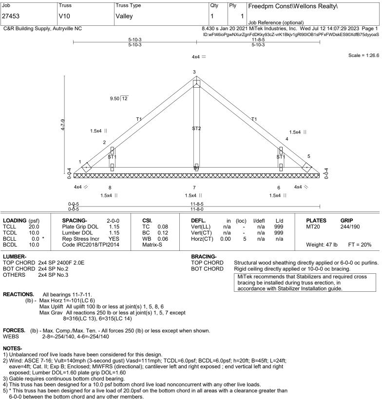
6) Provide mechanical connection (by others) of truss to bearing plate capable of withstanding 100 lb uplift at joint(s) 1, 5, 8,
