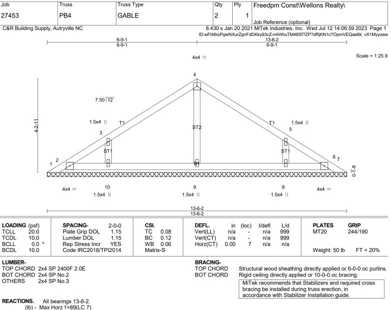
Max Uplift All uplift 100 lb or less at joint(s) 1, 7, 10, 8 Max Grav All reactions 250 lb or less at joint(s) 1, 7, 2, 6 except
