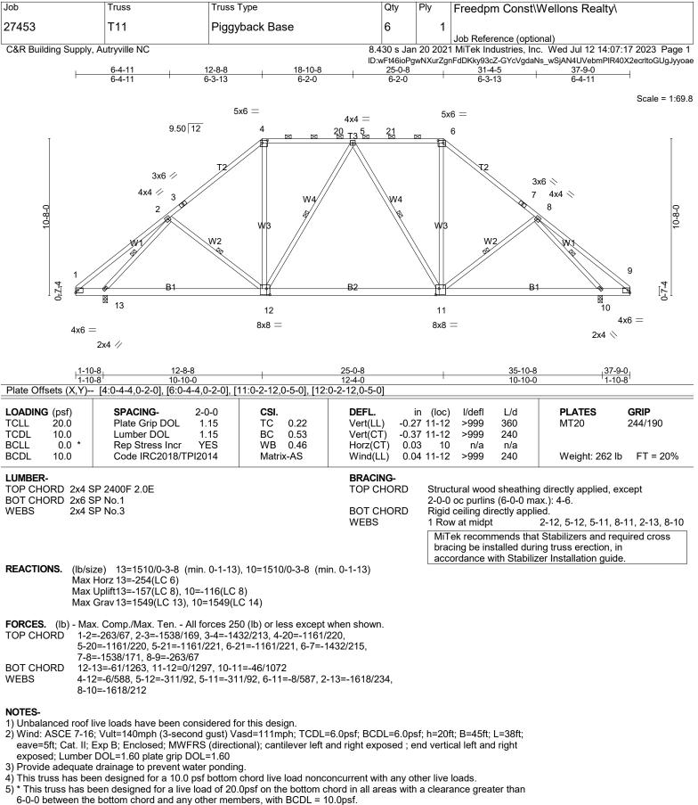
6) Provide mechanical connection (by others) of truss to bearing plate capable of withstanding 100 lb uplift at joint(s) except (jt=lb) 13=157, 10=116.
