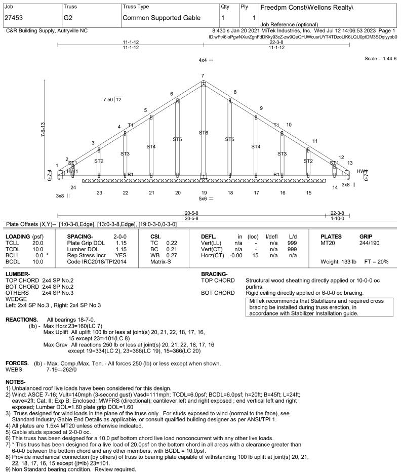
10) This truss is designed in accordance with the 2018 International Residential Code sections R502.11.1 and R802.10.2 and referenced standard ANSI/TPI 1.
