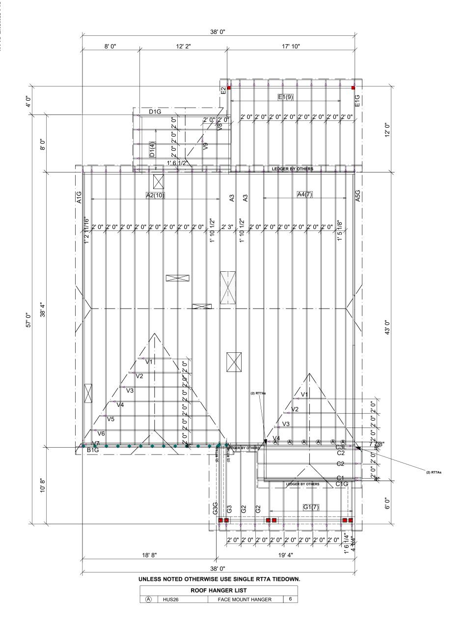
ROOF AREA: 2498.43 ft²\_RIDGE LINE: 68.93 ft \_ VALLEY LINES: 80.9 \_ HIP LINES:41.05 \_  $\triangle$  Indicates Left End of Truss
