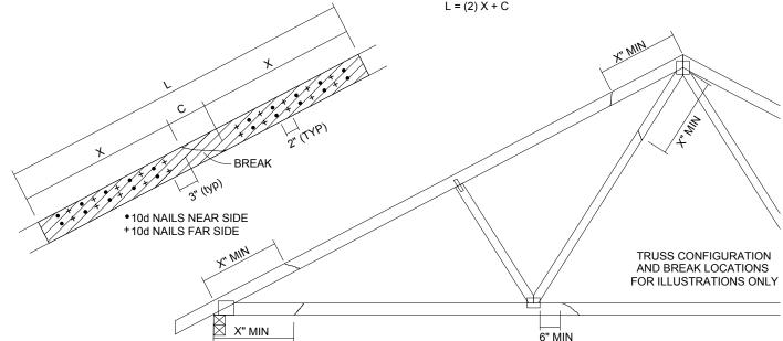
THE LOCATION OF THE BREAK MUST BE GREATER THAN OR EQUAL TO THE REQUIRED X DIMENSION FROM ANY PERIMETER BREAK OR HEEL JOINT AND A MINIMUM OF 6" FROM ANY INTERIOR JOINT (SEE SKETCH ABOVE)
