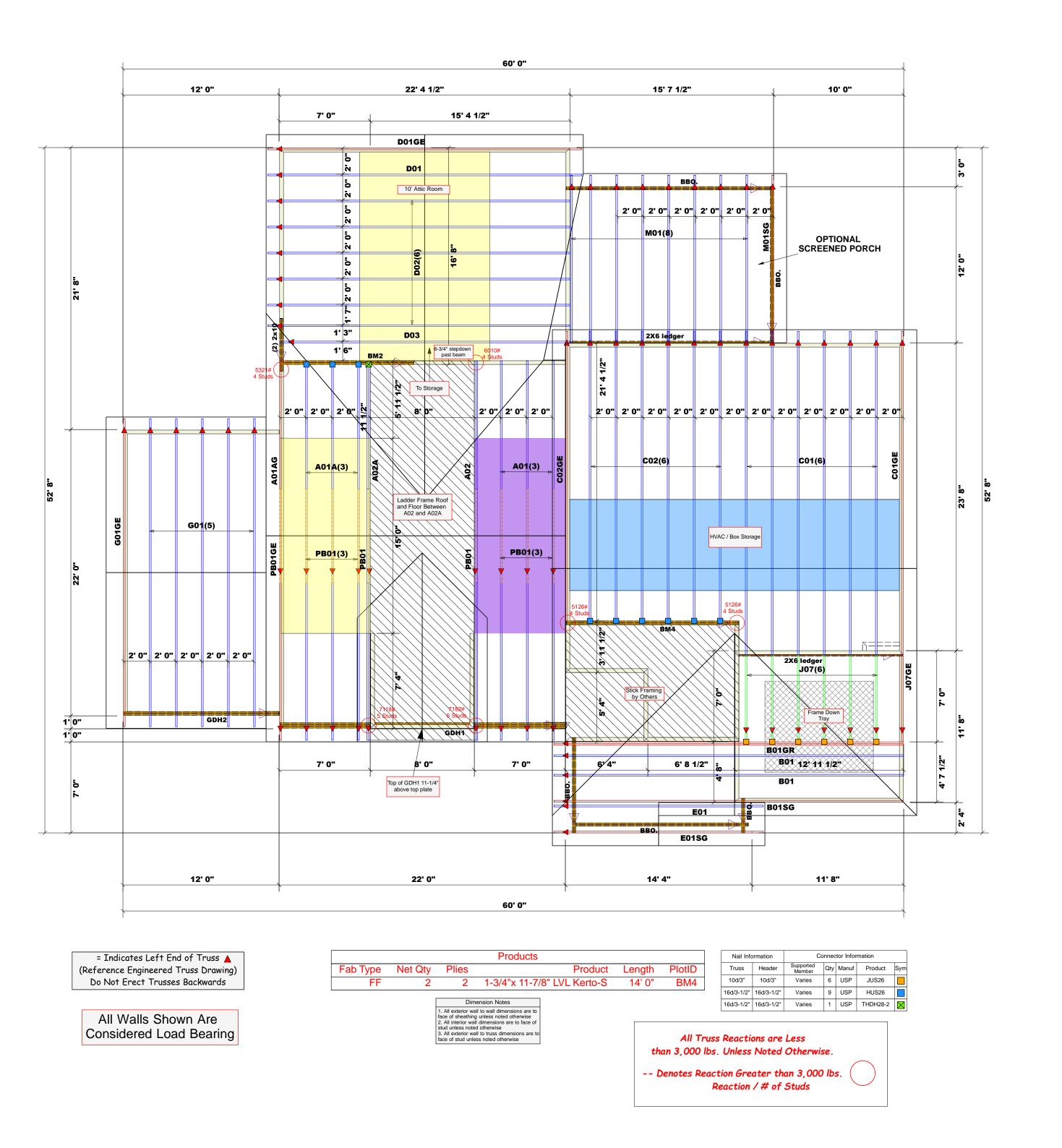
ROOF & FLOOR TRUSSES & BEAMS
