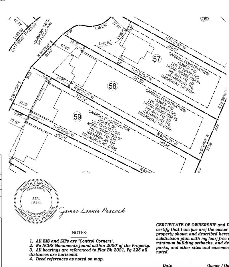
$\mathcal{L}EGEND$ POB Point of Beginning <sup>☉</sup> New Iron Set Iron Pin Found Wooden Bollard Found Stone Found Stake and Stone Ο **Cotton Spindle Set**  $\boxtimes$ Record Stone Not Found Property Lines ----- Fence Line Centerline of Road Edge of Asphault Woodline Edge of Concrete - E— Overhead Electric
