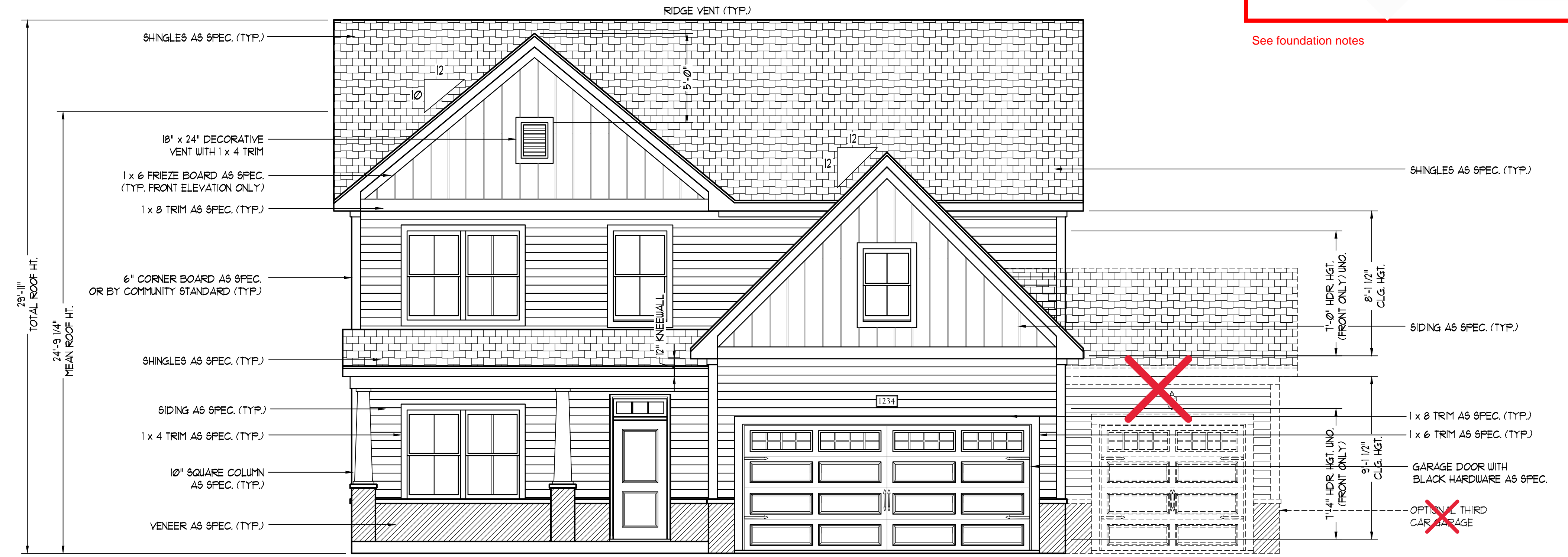
FRONT ELEVATION-B SCALE: 1/4" = 1'-0"
