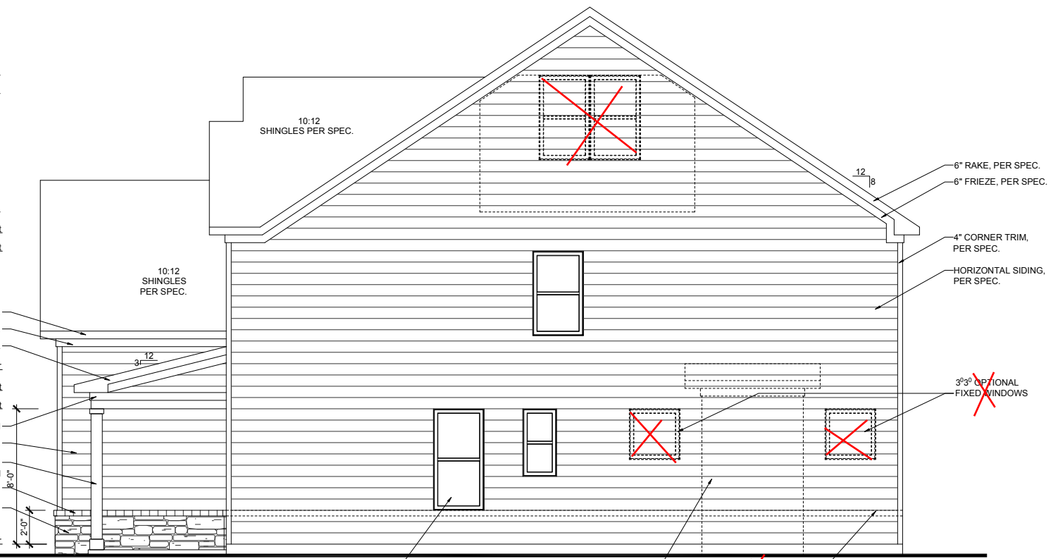
EXTENDED GARAGE RIGHT ELEVATION - A SCALE: 1/8"=1'-0" (11"x17" SHEET SIZE) SCALE: 1/4"=1'-0" (22"x34" SHEET SIZE)
