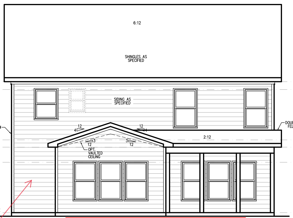
EXTENDED CAFE W/ COVERED PORCH REAR ELEVATION (SLAB) SCALE: 1/8"=1'-0" ON 11x17, 1/4"=1'-0" ON 22x34
