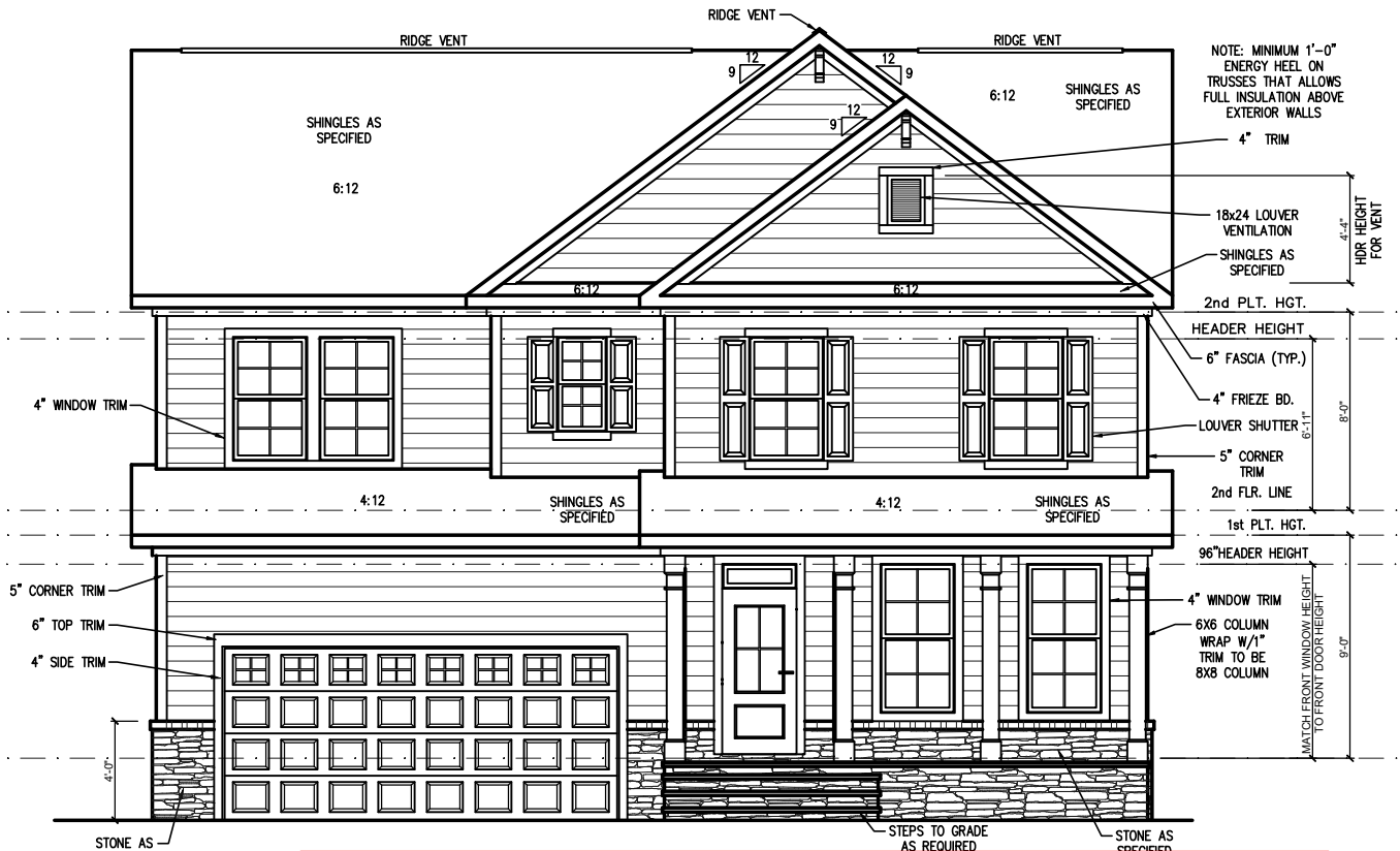
FRONT ELEVATION 'TRADITIONAL' (CRAWL/STEM WALL) SCALE: 1/4" = 1'-0" ON 22x34, 1/8" = 1'-0" ON 11x17 SEE FOUNDATION PAGES FOR FOUNDATION TYPE
