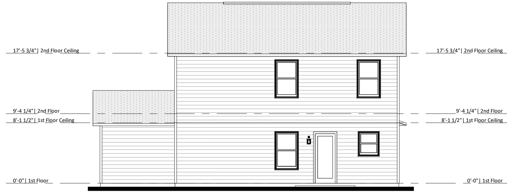
② Rear Elevation - Elev A - 2 Car Garage 1/8" = 1'-0"
