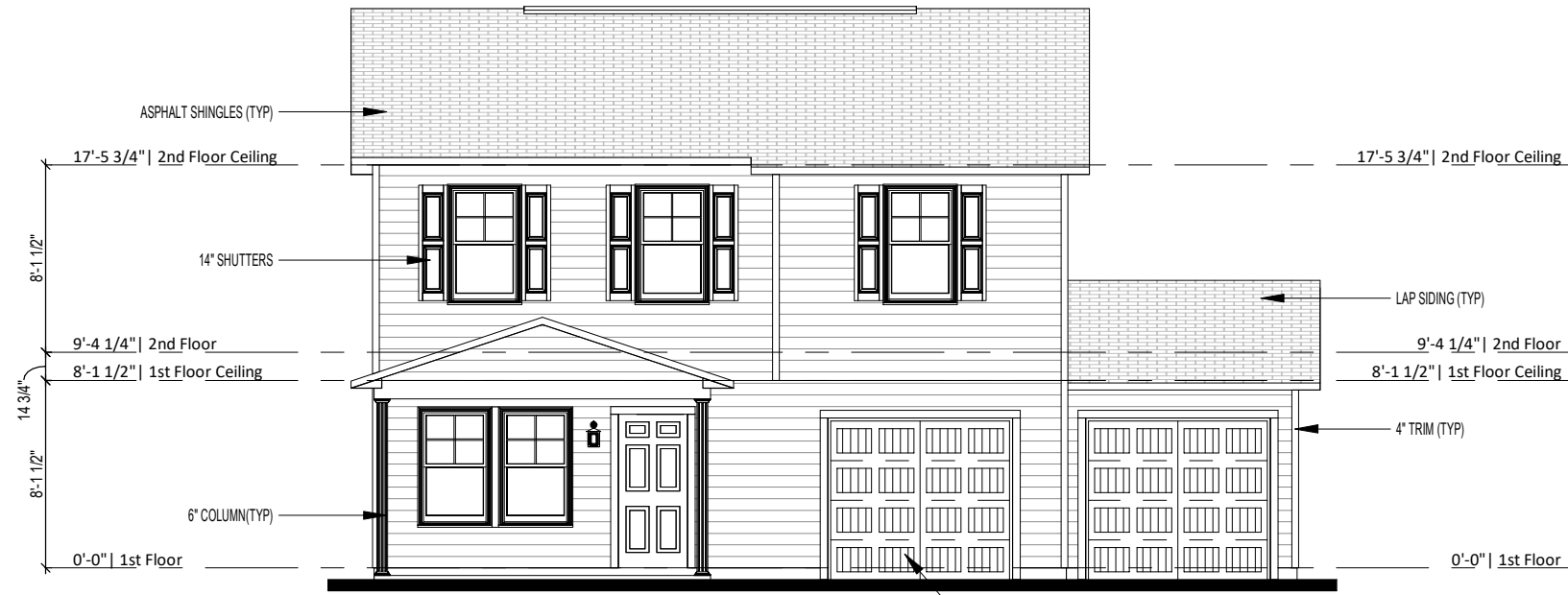
① Front Elevation - Elev A - 2 Car Garage 1/8" = 1'-0"
