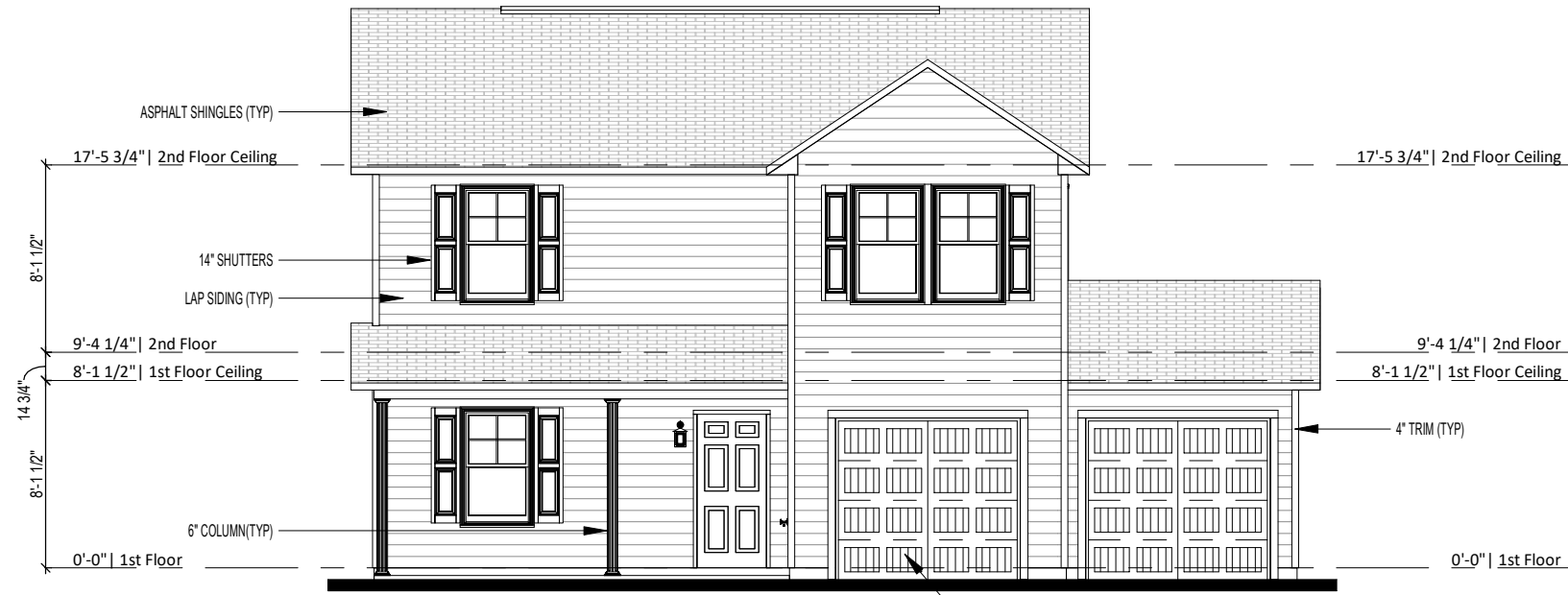
① Front Elevation - Elev A - 2 Car Garage 1/8" = 1'-0"
