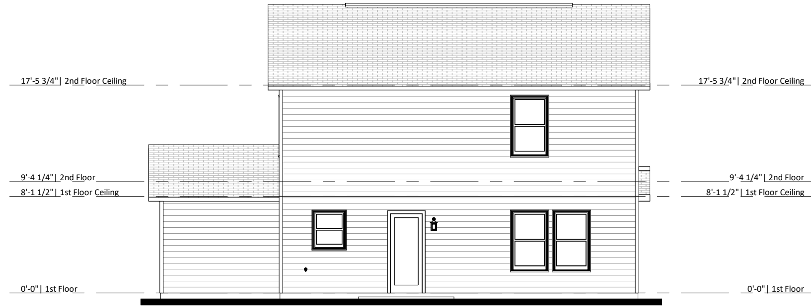
② Rear Elevation - Elev A - 2 Car Garage 1/8" = 1'-0"
