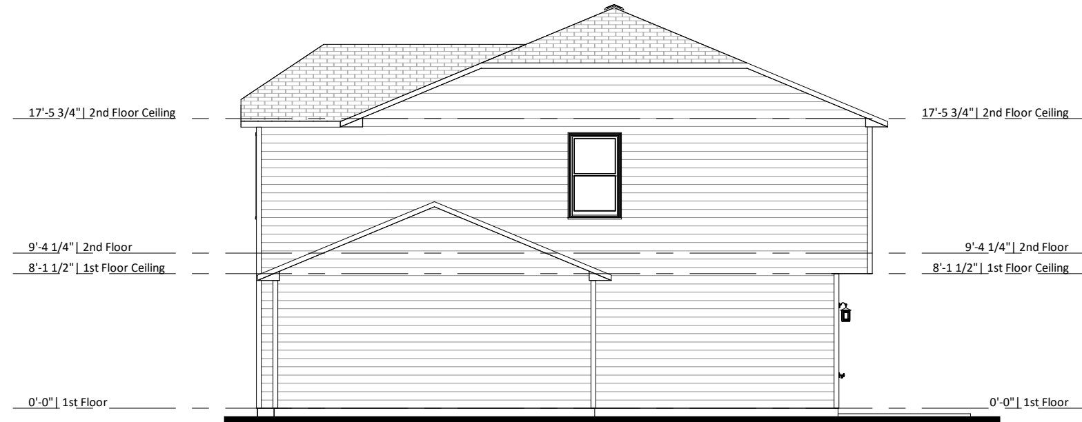
① Right Elevation - Elev B - 2 Car Garage 1/8" = 1'-0"
