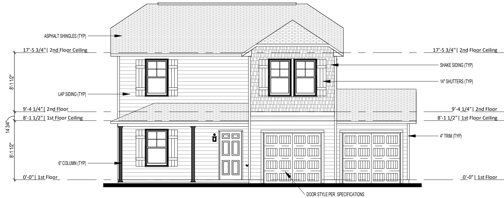
① Front Elevation - Elev B - 2 Car Garage 1/8" = 1'-0"
