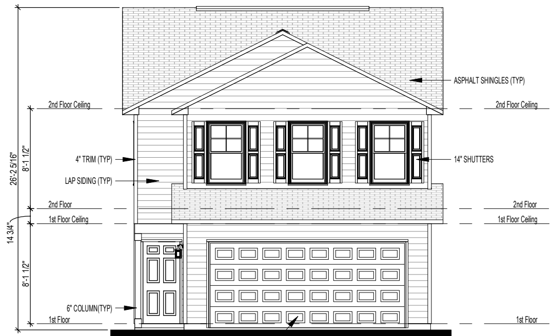
1 Front Elevation - Elev A 1/8" = 1'-0"
