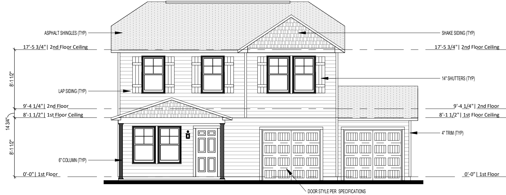
① Front Elevation - Elev B - 2 Car Garage 1/8" = 1'-0"
