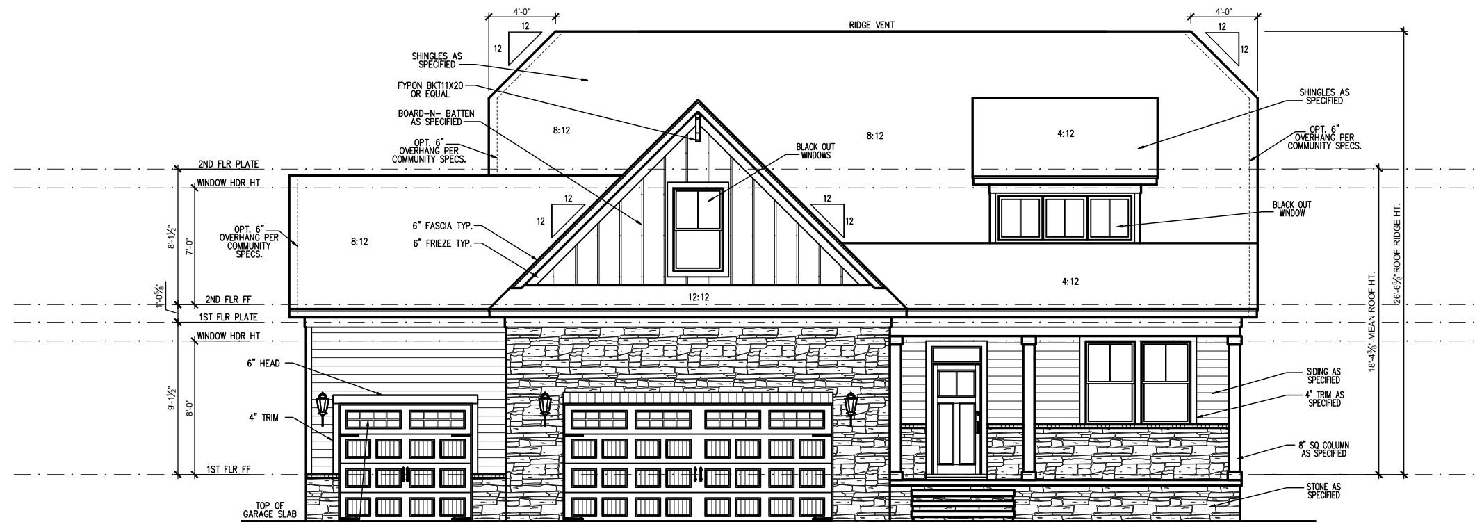
FRONT ELEVATION 'B' - 3 CAR FRONT LOAD SCALE: 1/8"=1'-0" ON 11x17, 1/4"=1'-0" ON 22x34
