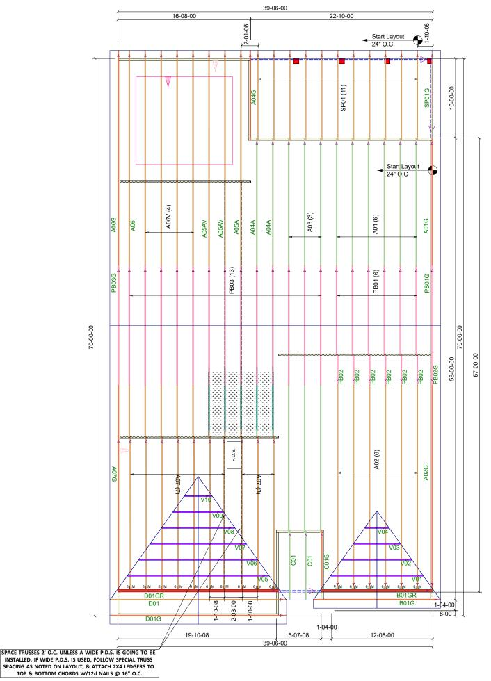
SPACE TRUSSES 2' O.C. UNLESS A INSTALLED. IF WIDE P.D.S. IS U SPACING AS NOTED ON LAYOUT
