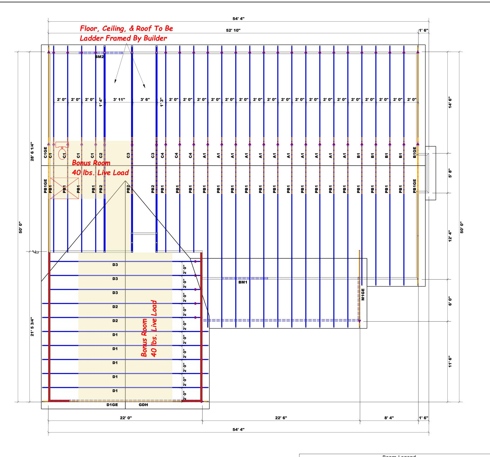
Truss Placement Plan SCALE: 1/4" = 1'
