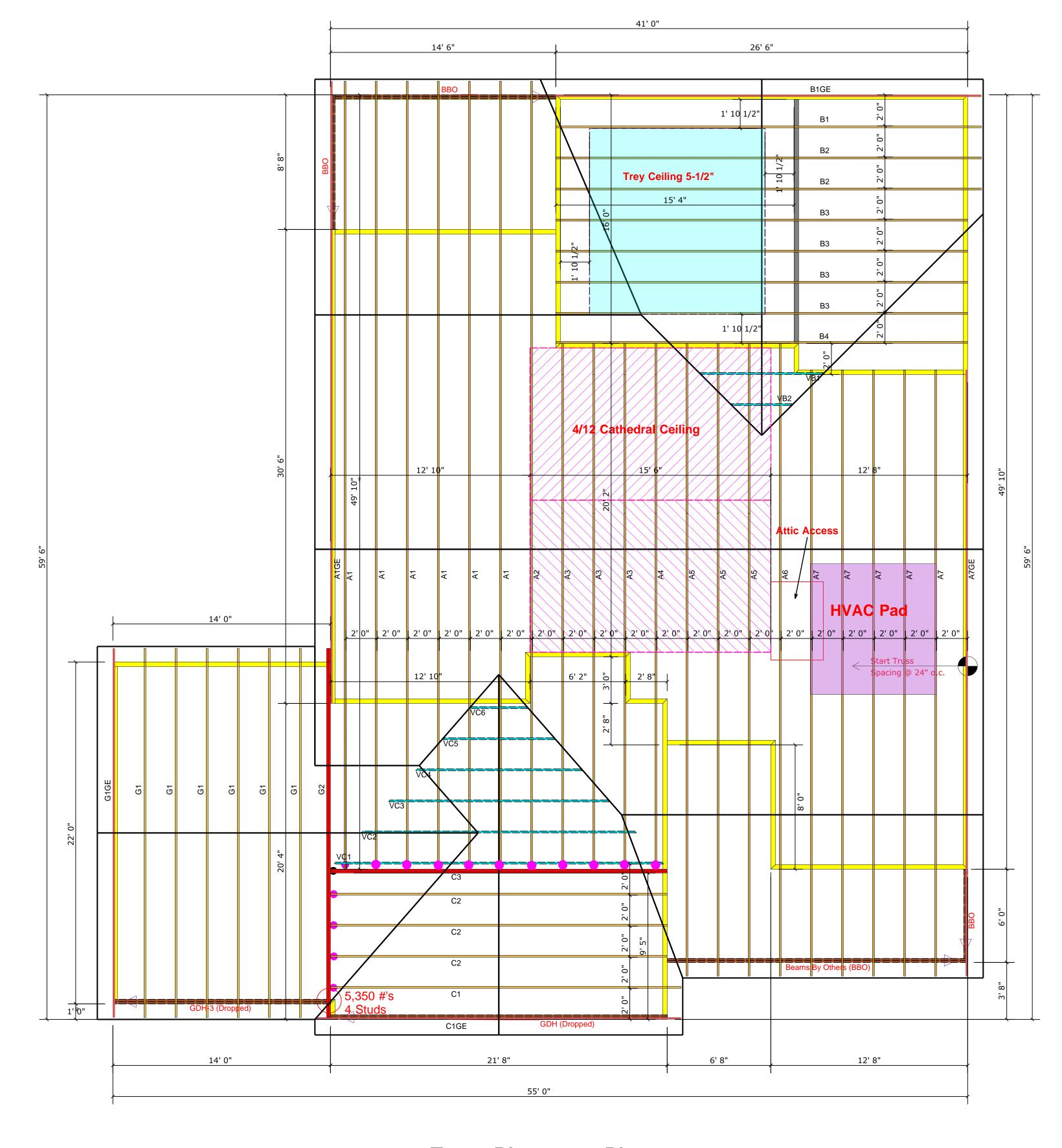
Truss Placement Plan SCALE: 1/4" = 1'-0"
