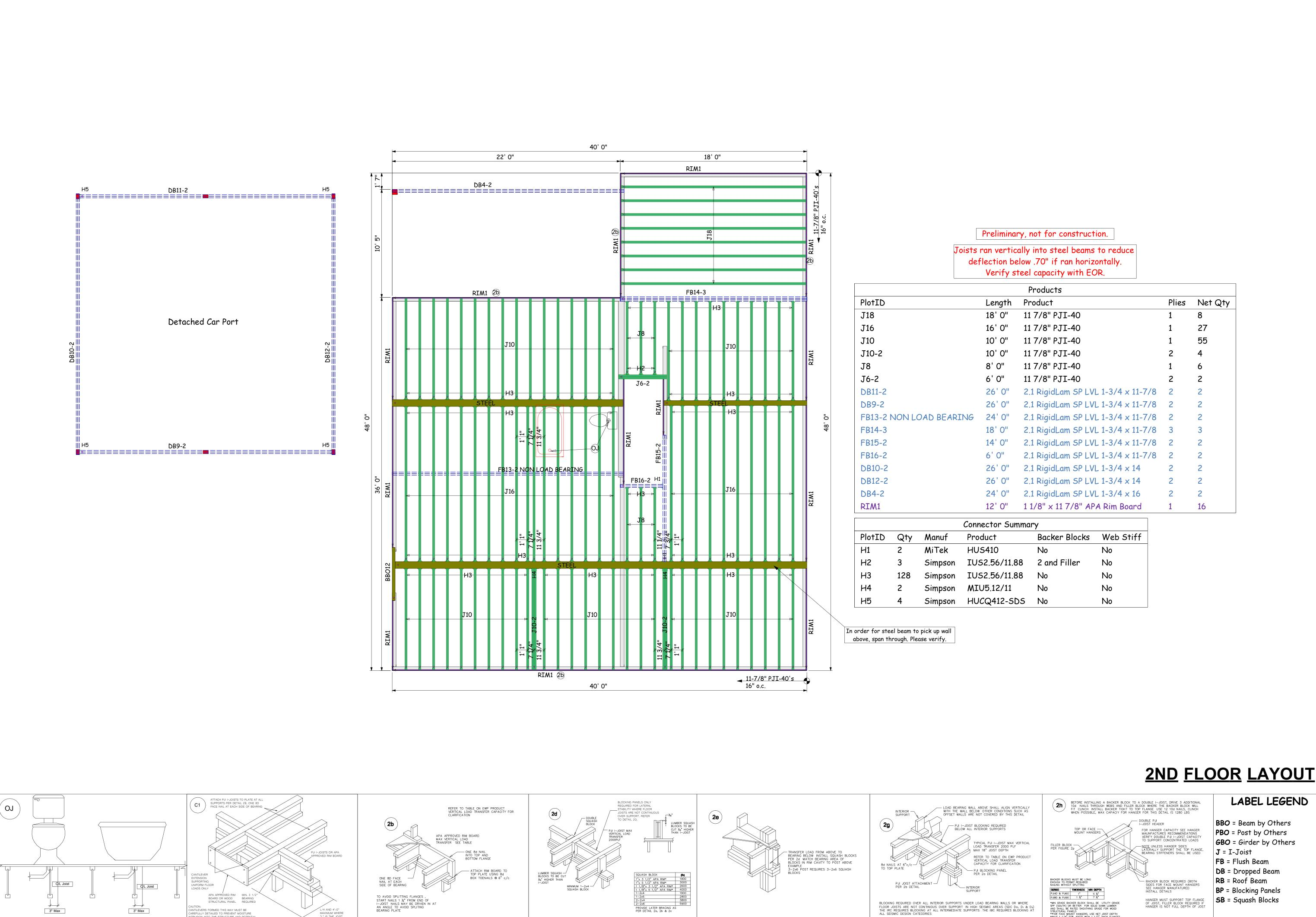
ALL POINT LOADS FROM ABOVE MUST BE TRANSFERRED TO BEARING FROM UNDER SIDE OF SHEATHING.
