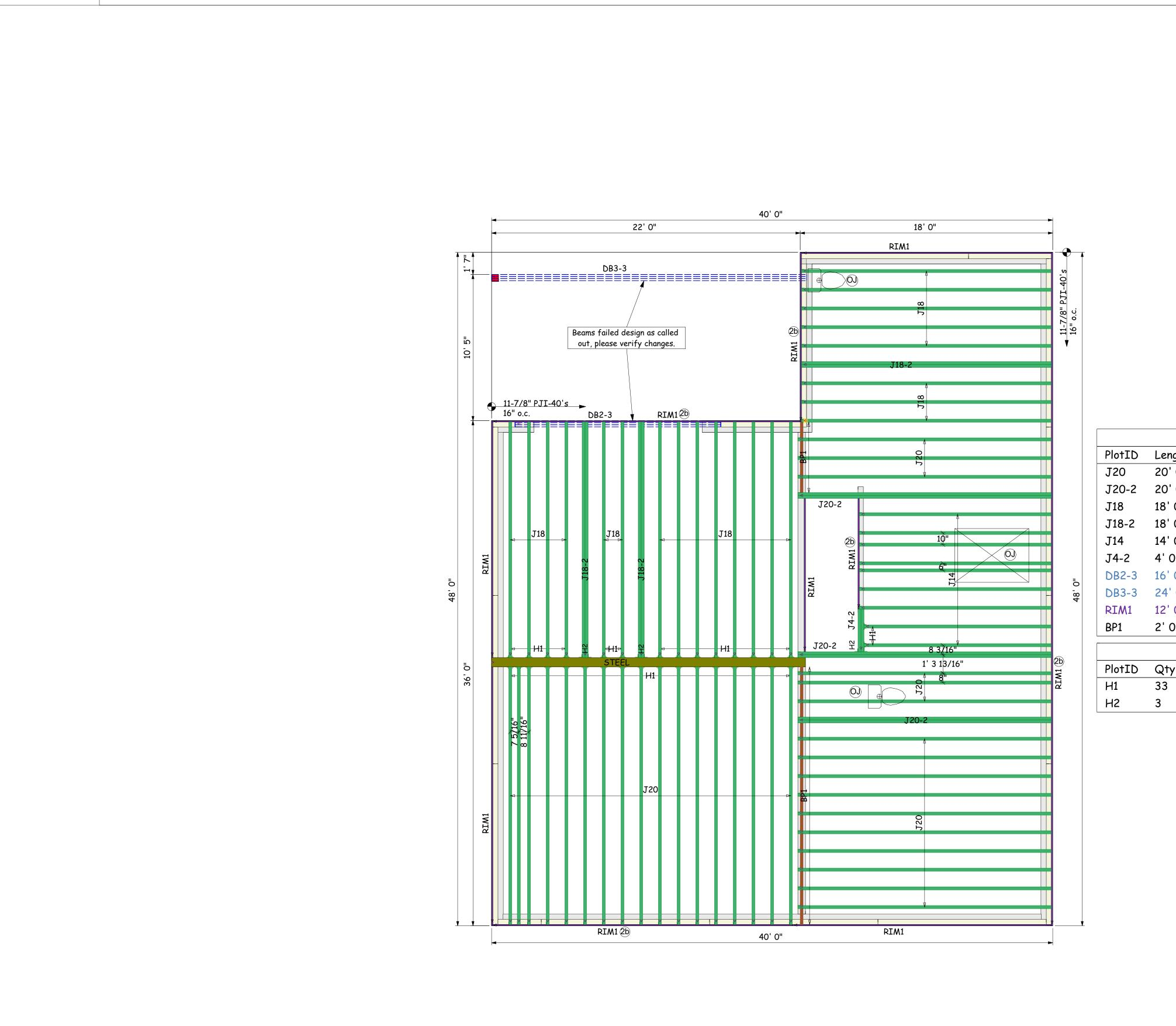
General Notes: \*\* CUTTING OR DRILLING OF COMPONENTS SHOULD NOT BE DONE WITHOUT CONTACTING COMPONENT SUPPLIER FIRST. CUSTOMER TAKES FULL RESPONSIBILITY FOR COMPONENTS IF CUT BEFORE AUTHORIZATION.
