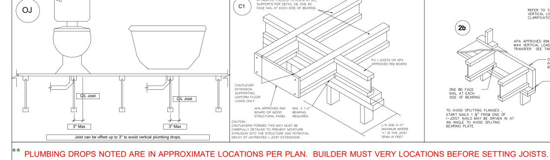
ATTACH PJII I-JOISTS TO PLATE AT ALL SUPPORTS PER DETAIL 2B, ONE 8D FACE NAIL AT EACH SIDE OF BEARING
