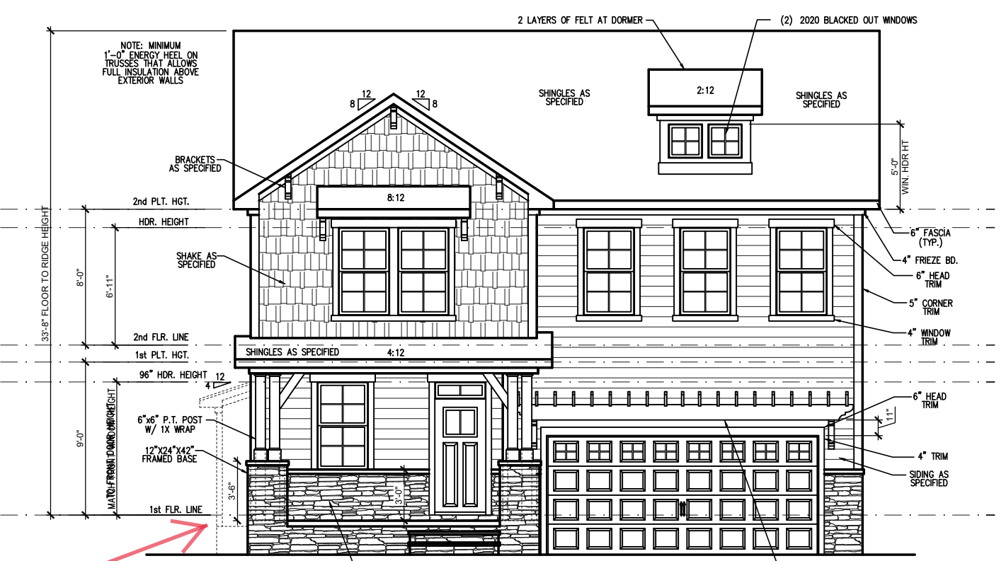
FRONT ELEVATION 'ENGLISH COUNTRY' (CRAWL/STEM WALL) SCALE: 1/4" = 1'-0" ON 22x34, 1/8" = 1'-0" ON 11x17 SEE FOUNDATION PAGES FOR FOUNDATION TYPE
