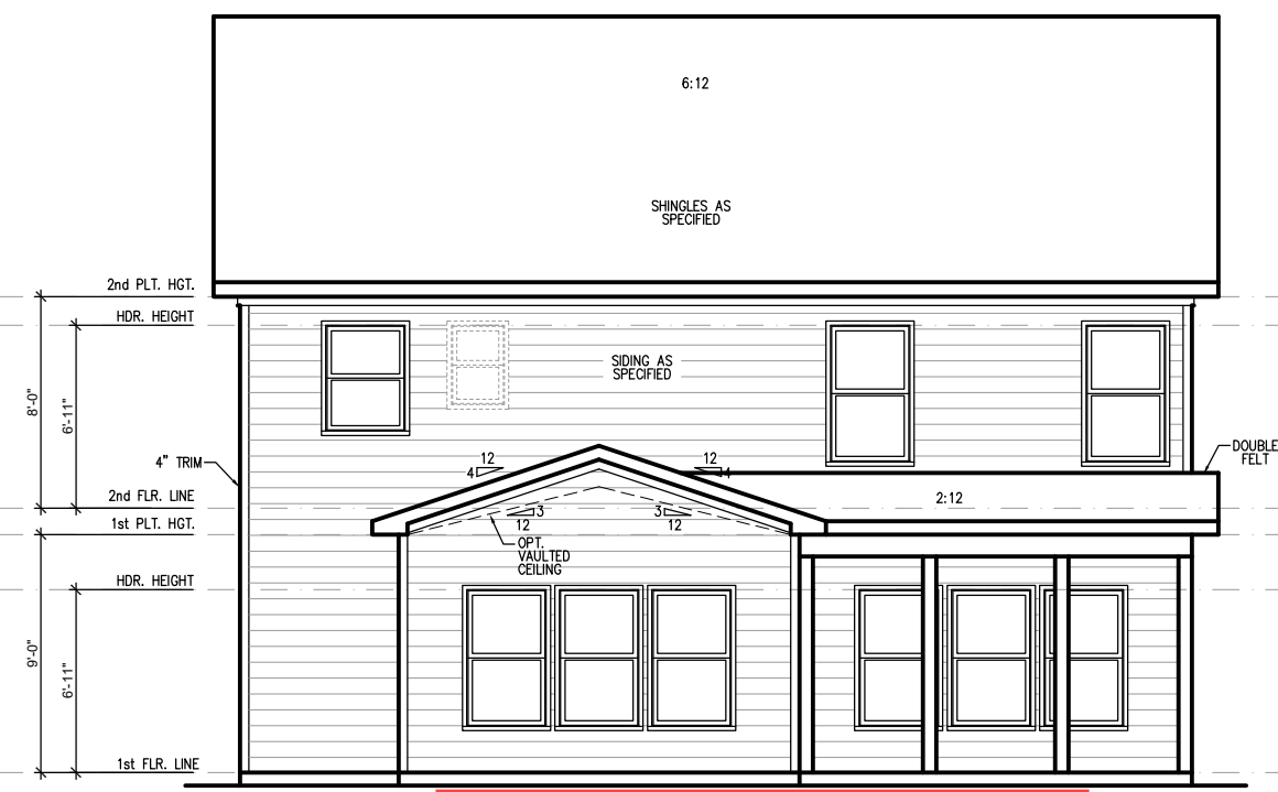
EXTENDED CAFE W/ COVERED PORCH REAR ELEVATION (SLAB) SCALE: 1/8"=1'-0" ON 11x17, 1/4"=1'-0" ON 22x34
