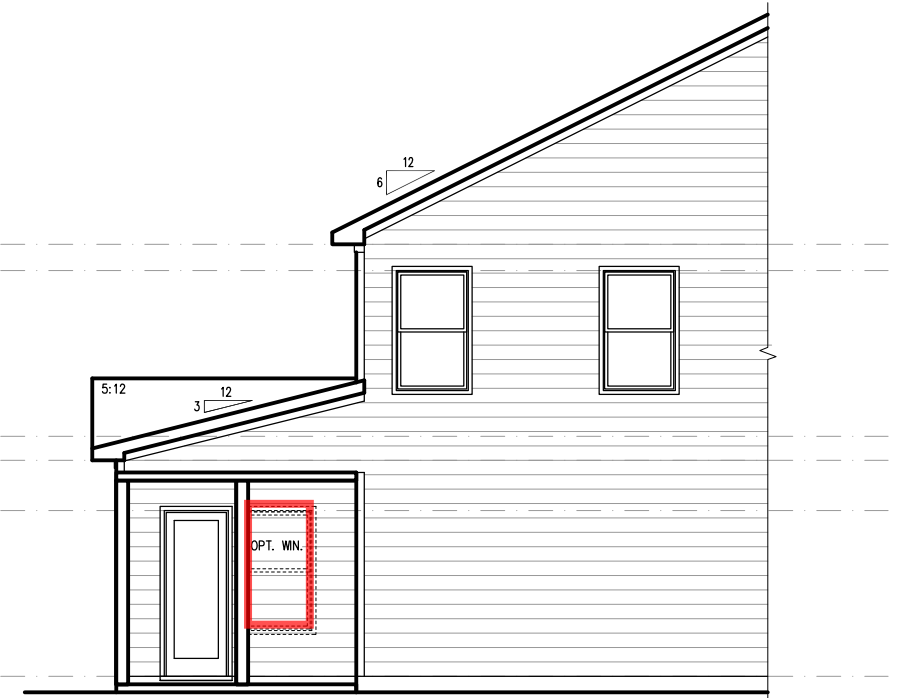
EXTENDED CAFE W/ COVERED PATIO PARTIAL RIGHT SIDE ELEVATION (SLAB) SCALE: 1/8"=1'-0" ON 11x17, 1/4"=1'-0" ON 22x34
