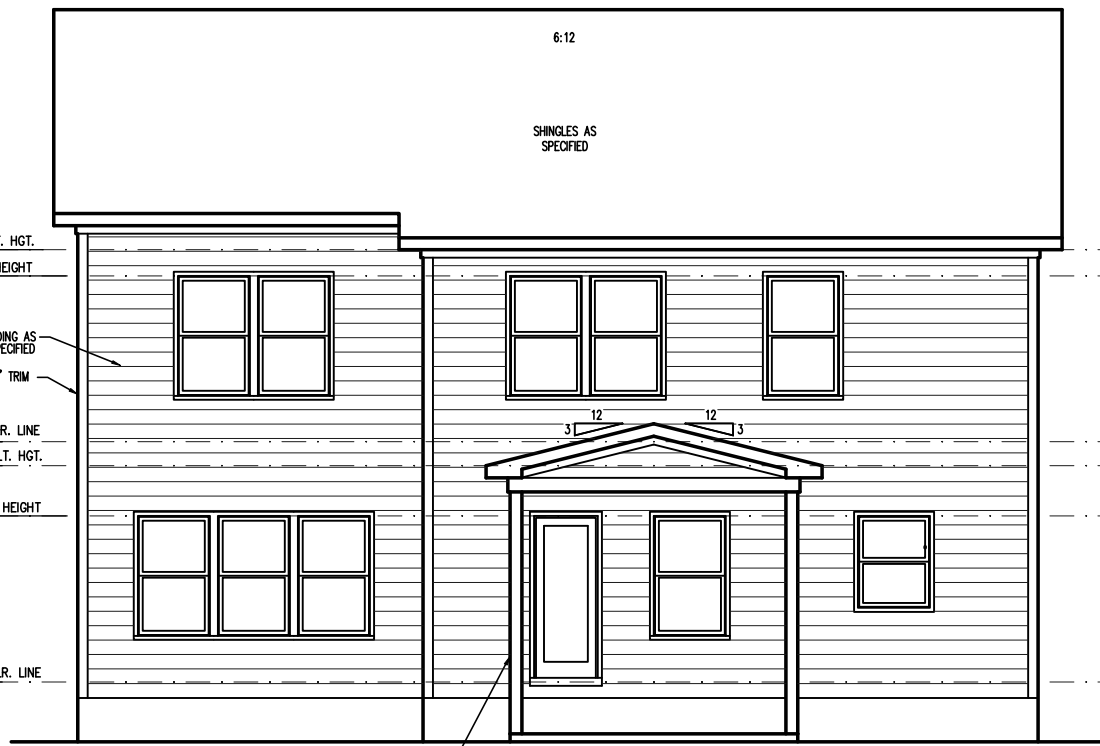
COVERED PATIO REAR ELEVATION (CRAWL)
