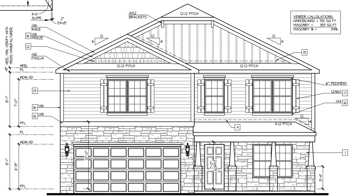
Front Elevation 'C' SCALE: 1/4"=1'-0" AT 22"x34" LAYOUT 1/8"=1'-0" AT 11"x17" LAYOUT
