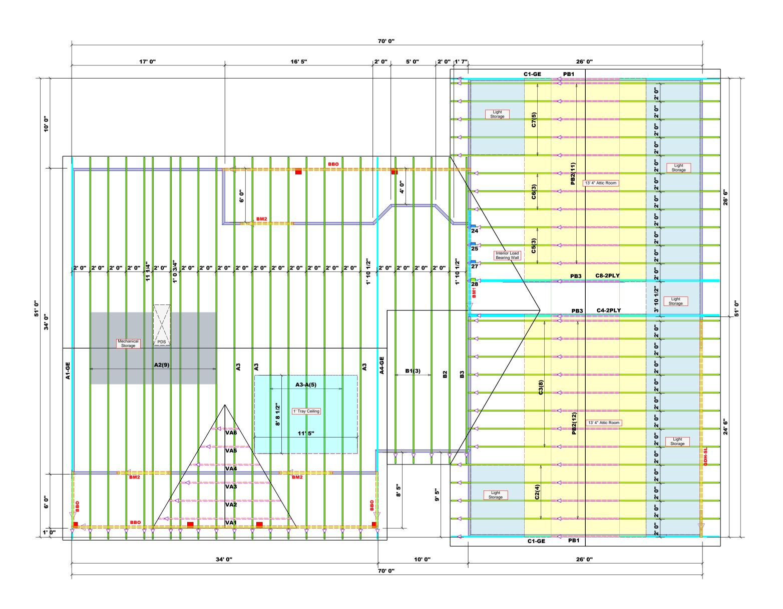
▲ = Indicates Left End of Truss (Reference Engineered Truss Drawing) Do Not Erect Trusses Backwards
