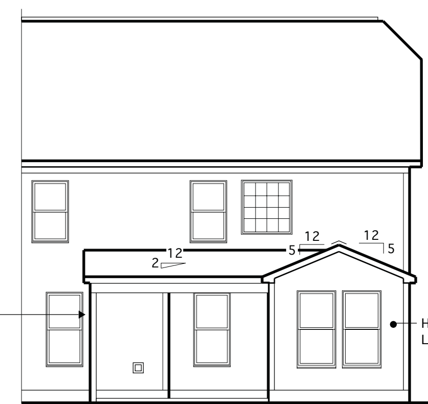
REAR ELEV. W/ OPT. SUNROOM & OPT. COVERED PORCH SCALE: 1/8"=1'-0" NOTE: SEE SHEET 4.1 FOR OPT. SUNROOM & OPT. COVERED PORCH W/ ALT. FIREPLACE LOCATION
