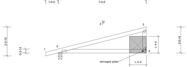
Repair for a damaged plate as shown.
