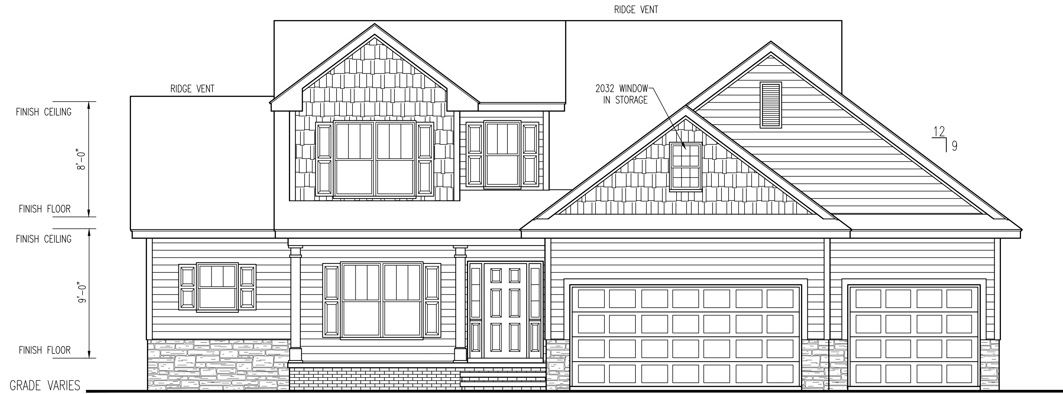
FRONT ELEVATION SCALE: 1/4" = 1'-0"
