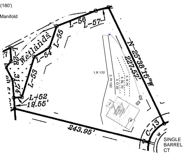
preliminary septic plan made prior to final construction activities. A revised plan may need to be reworked at time of permitting.
