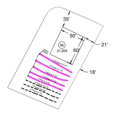
System: Gravity to Serial Dist. Lines: 1-5, (375')
