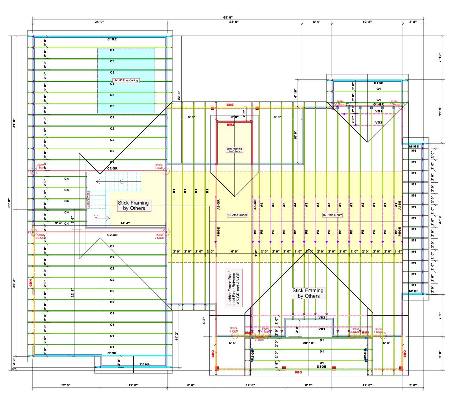
All Truss Reactions are Less than 3,000 lbs. Unless Noted Otherwise -- Denotes Reaction Greater than 3,000 lbs. Reaction / # of Studs
